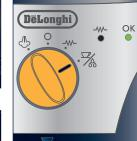
When OK light is green, turn dial to by position to start coffee delivery. And when the desired amount is reached, turn back to -W- position to stop.
